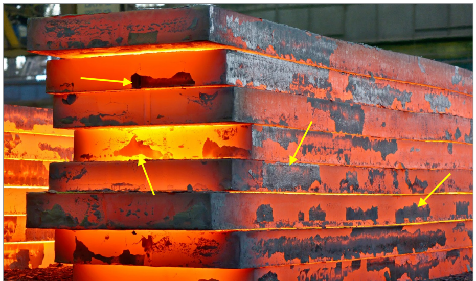
Figure 4.0 - Steel plates minutes after manufacturing. The arrows showcase scale (iron oxides) produced by dry corrosion. This is a natural process that transforms the “non-natural” material (steel) back to a mineral.
